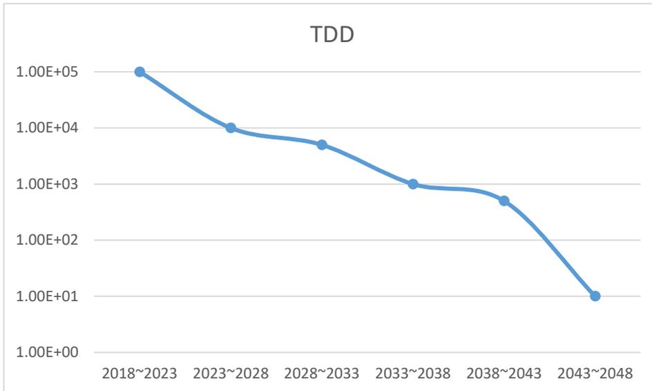
Fig 1.23 Development trend of the TDD of GaN substrate
