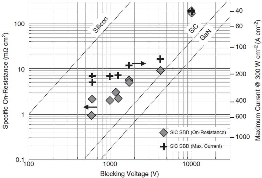
Fig 1.7 The development of SiC Schottky device
