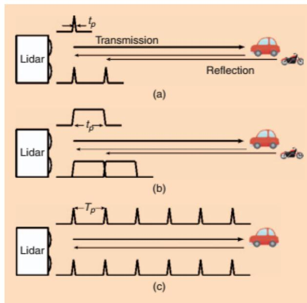
**Figure 4.12 Influence of lidar pulse width on distance measurement resolution**
