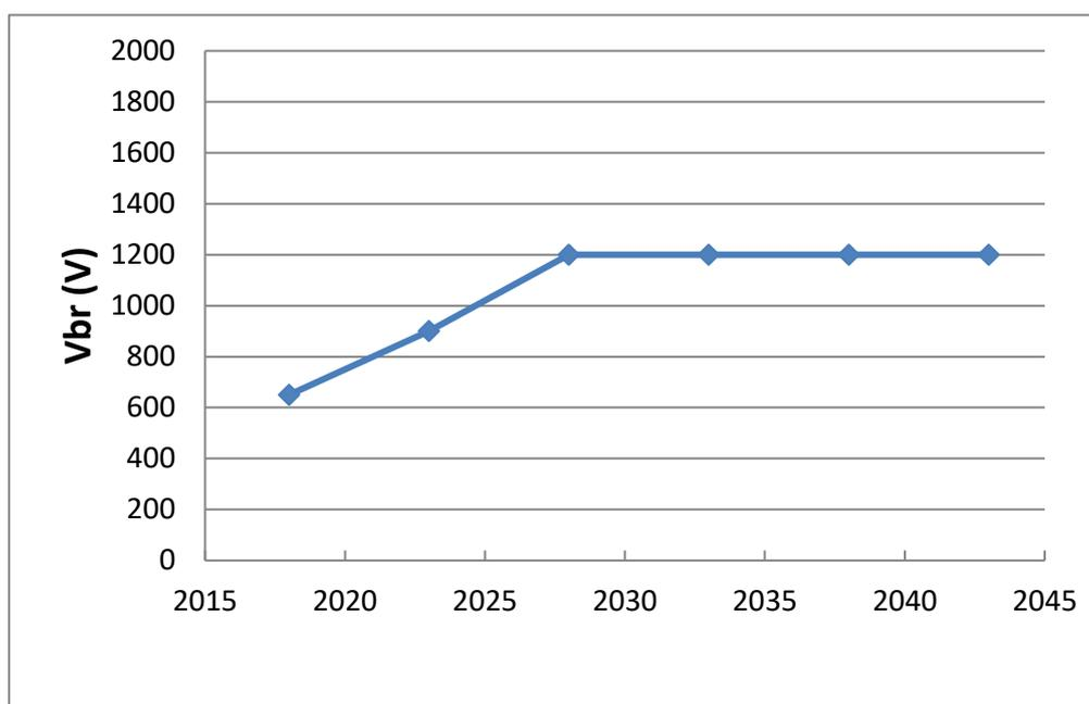
Fig 1.18 Development trend of withstand voltage level of Si-based GaN power electronic devices
