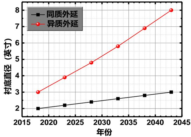
Fig 1.29 Development trend of the size of the diamond substrate
