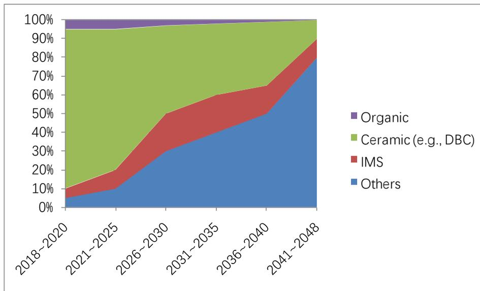
Fig. 2.16 The application trend of substrate in inverter for motor driving application
