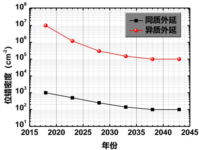
Fig 1.30 Development trend of diamond substrate defect density
