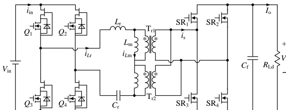
**Figure 4.6 Main circuit structure diagram of the prototype**
