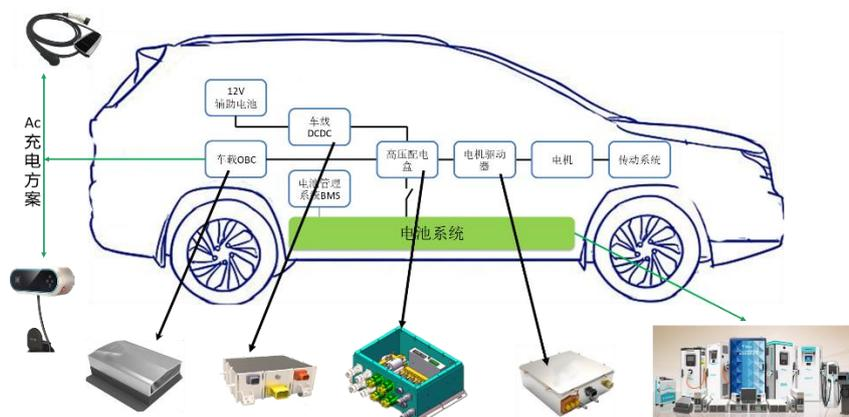
**Figure 3.1 Electric vehicle and power electronic device**
