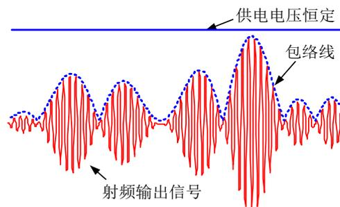
**Figure 4.14 Typical waveform for constant voltage supply**
