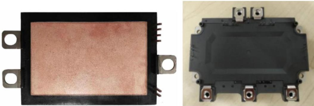
Fig.2.2 Typical structure of MOSFET adopting SiC device
