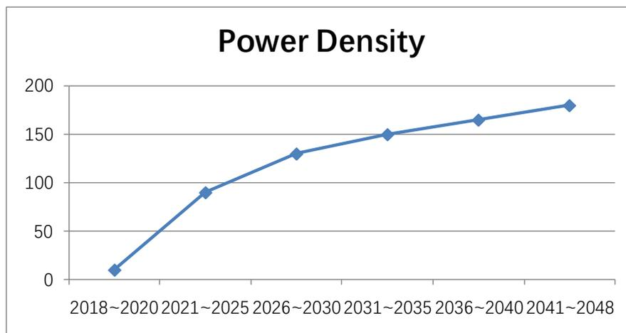
Fig. 2.11 The power density trend of SiC-MOSFET in inverter for motor driving application( $\text{W}/\text{cm}^3$ )
