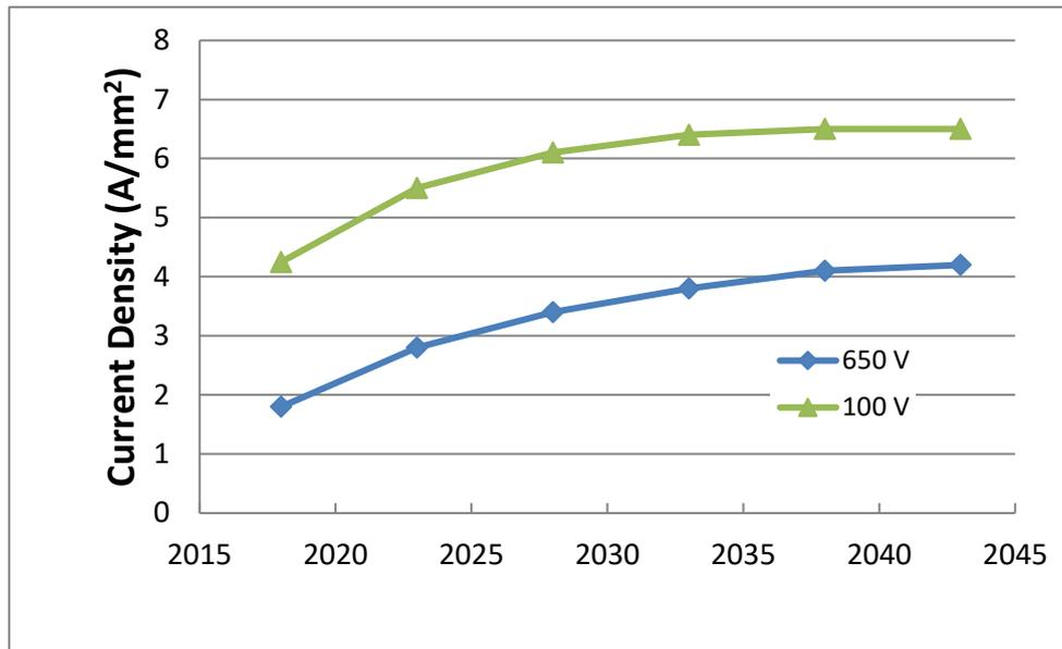
Fig 1.20 Current trends in GaN power electronics current density
