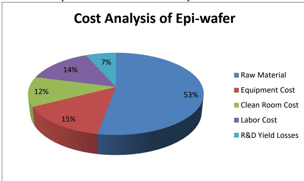
Fig 1.5 Cost analysis of epitaxial wafers
