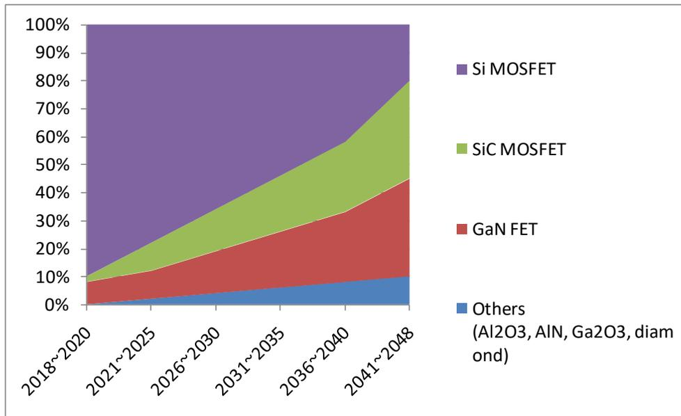
Fig. 2.12 The application trend of power device in DC-DC converter
