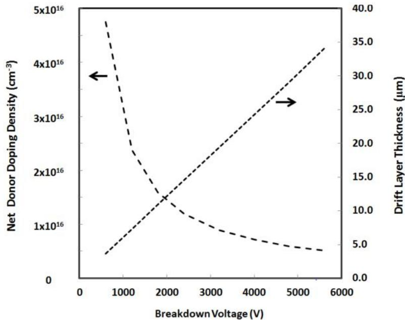
Fig 1.25 The relationship between epitaxial thickness, the doping concentration in the drift region and the breakdown voltage of GaN
