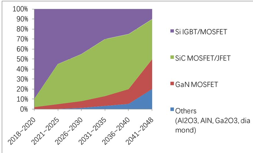
Fig. 2.15 The material of power device in inverter for motor driving application
