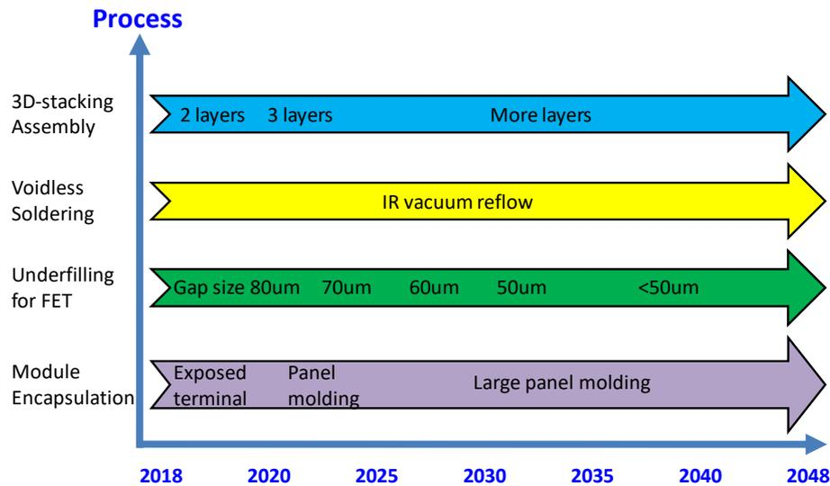
Fig. 2.14 The application trend of packaging and integration process for DC-DC converter
