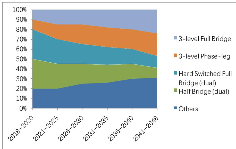
Fig. 2.8 The topology development trend of SiC-MOSFET in inverter for motor driving application
