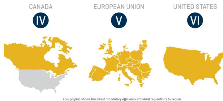
**Figure 3.5 Energy efficiency standard requirements for adapter power products**
