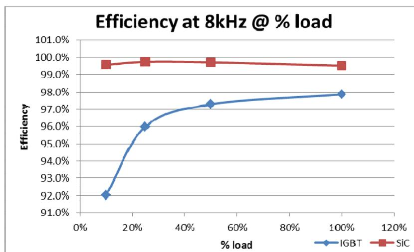
**Figure 2.3 Efficiency comparison between Si IGBT and SiC MOSFET controllers**
