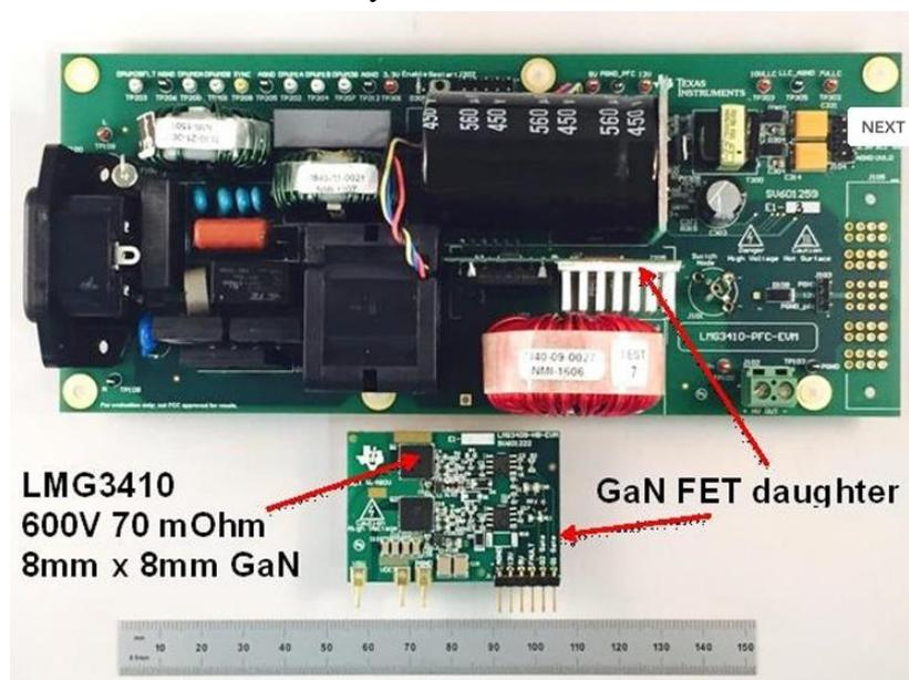
**Figure 4.10 TI's power master based on GaN device PFC (source: TI website)**
