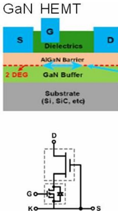
Figure 4.1 Cascode GaN transistor
