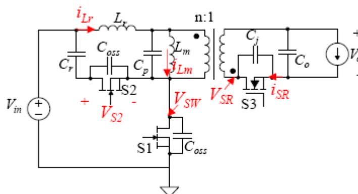
**Figure 4.9 Circuit diagram of the active clamped flyback converter**
