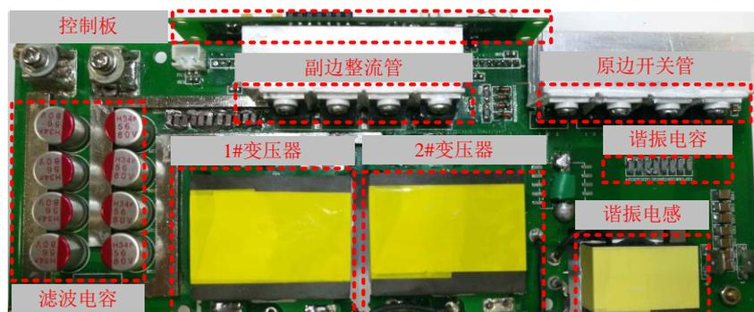
**Figure 4.7 Photo of the prototype**
