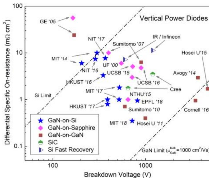
Fig 1.27 Comparison of GaN p-n diodes with other diodes.
