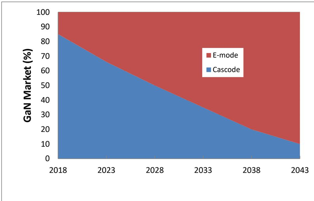
Fig 1.19 Development trend of market share of different device structures in the GaN power electronics
