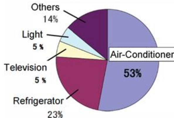
Figure 3.7 Power consumption distribution of different household electronic
