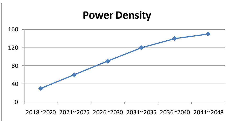
Fig. 2.10 The trend of power density of DC-DC converter ( $\text{W}/\text{cm}^3$ )
