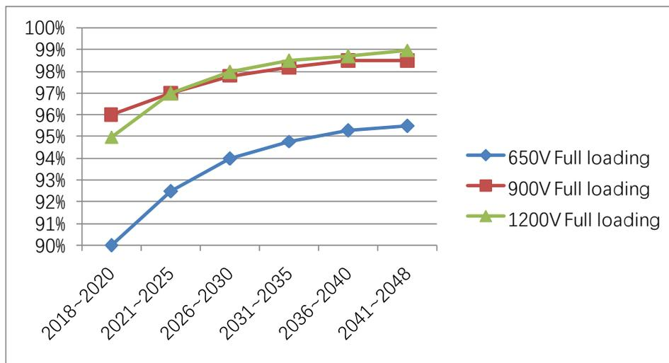
Fig.2.9 The conversion efficiency trend of SiC-MOSFET in inverter for motor driving application
