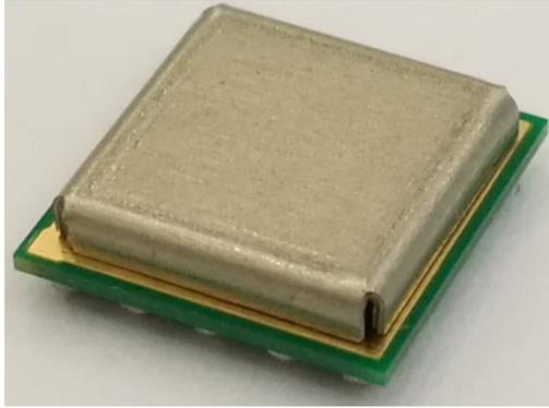
Fig. 2.1 Typical structure of DC-DC converter adopting GaN device
