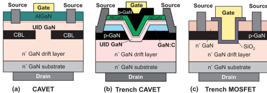
Fig 1.28 Structure diagram of the GaN transistor
