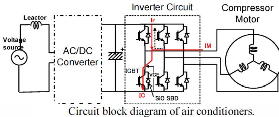
**Figure 3.8 Block diagram of air conditionings electrical control system**
