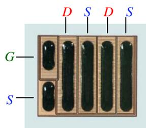
Figure 4.2 Schematic diagram of LGA package
