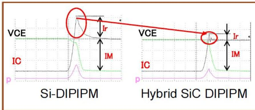
Figure 3.10 Comparison of turn-on voltage/ current waveforms
