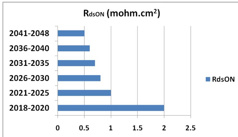
Fig 1.13 The specific on-resistance of SiC MOSFET
