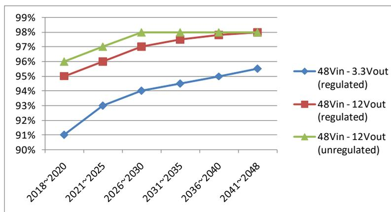
Fig. 2.7 The trend of conversion efficiency of DC-DC converter
