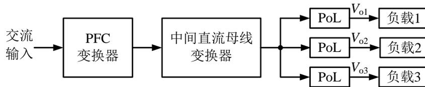
Figure 4.5 Structure of distributed server power system
