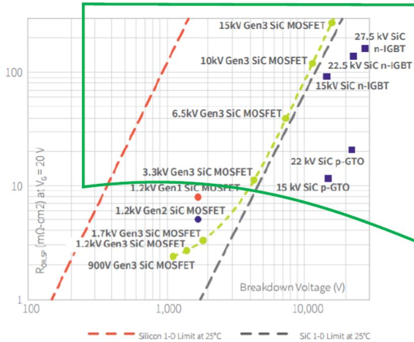
Fig 1.12 Current current voltage level of SiC MOSFET
