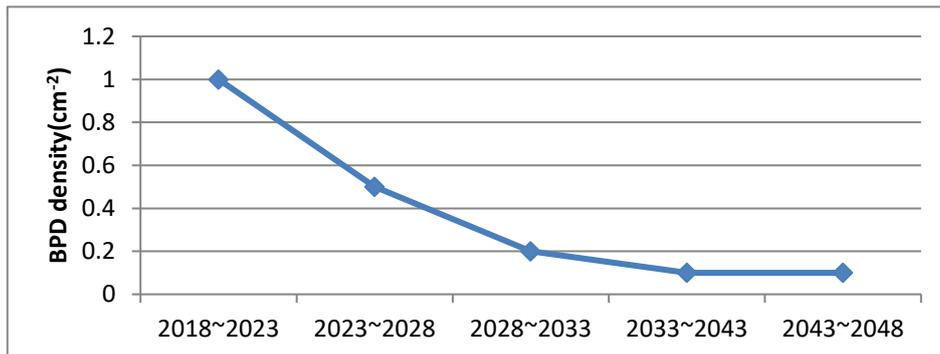
Fig 1.4 The development trend of BPD density in SiC epitaxial wafer
