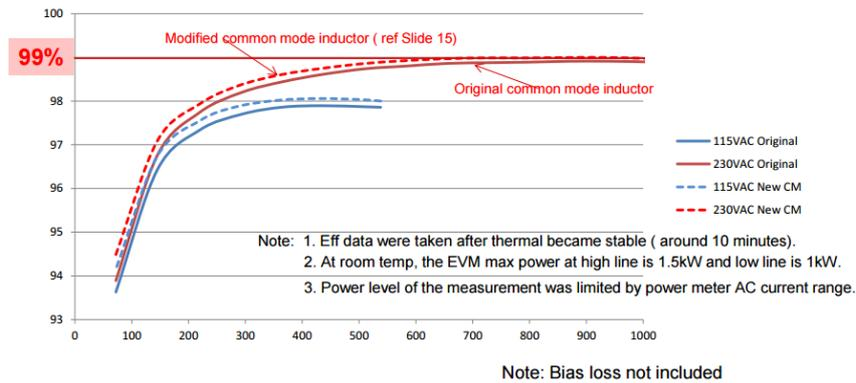
**Figure 4.11 TI's PFC efficiency changes with power based on GaN devices (source: TI website)**
