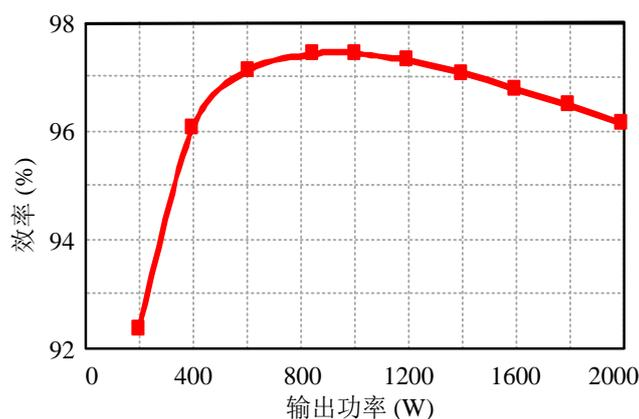
**Figure 4.8 Efficiency curve as a function of load**
