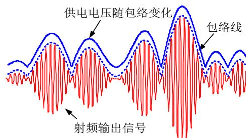
**Figure 4.15 Typical waveform of the envelope following the power supply**
