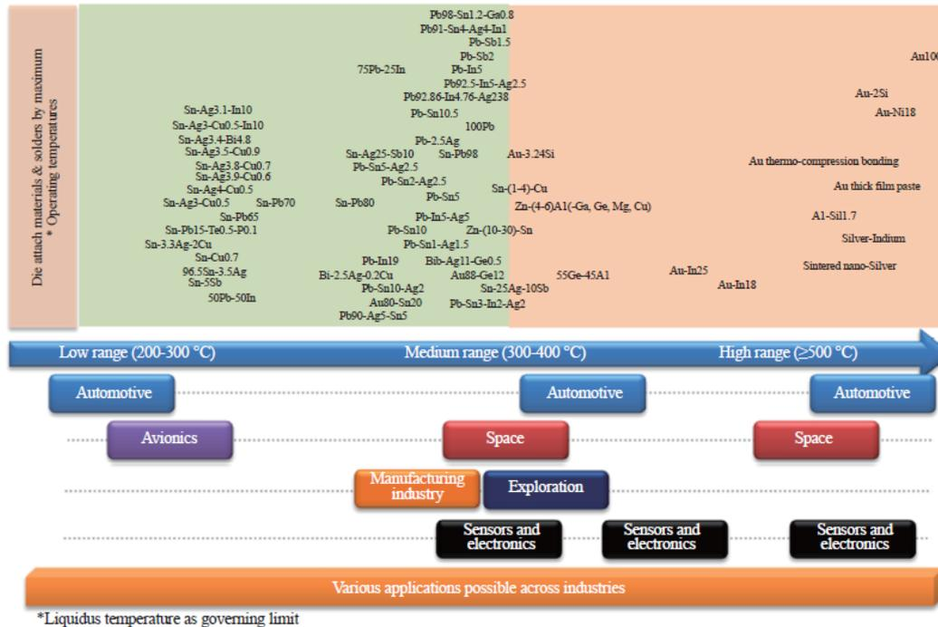
Fig 1.16 Materials that can be used in SiC power device packages in the future
