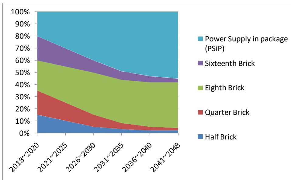
Fig.2.3 The application trend of DC-DC converter of various dimensions
