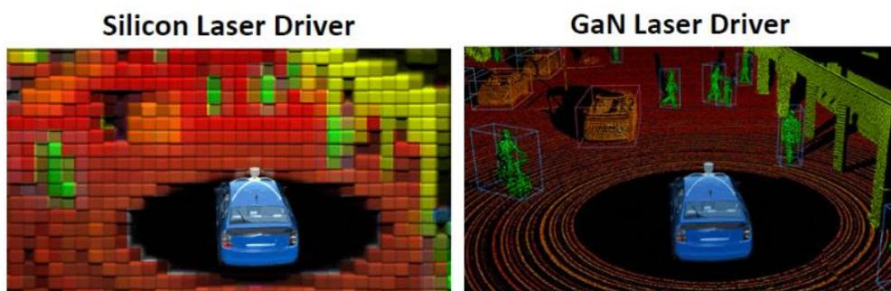
**Figure 4.13 Comparison of lidar imaging resolution driven by Si and GaN devices (source: US EPC Corporation )**
