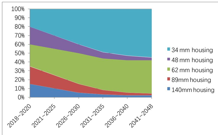
Fig. 2.4 The dimension trend of SiC-MOSFET in inverter for motor driving application
