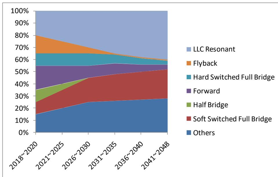
Fig. 2.5 The trend of topology in DC-DC converter
